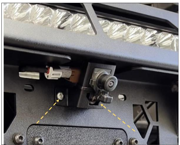
19. Secure the camera bracket to the mesh panel using supplied M4 screws, washers and flange nuts.
